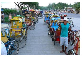
The word "sikad" means kick or pedal, so it's unclear if its meaning comes from pedaling the bicycle or when the driver kicks the foot brake on the front wheel. The brake is one of the most interesting feature of this type of Philippines pedicab as it's simply a foot brake on a sprung hinge over the front wheel, with a piece of car tire used as the brake onto the rubber bicycle tire.
